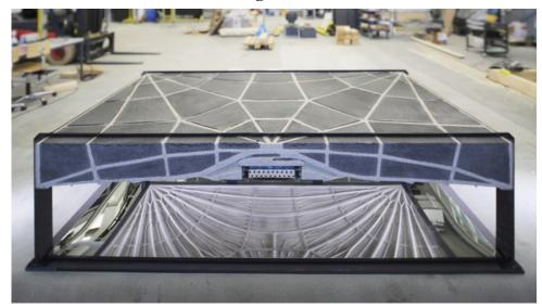
Figure 49: 3D Printed Formwork for Integrated Funicular Concrete Slabs
